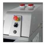
**Two three-phase power sockets**Facilitates the connection of moulder and divider.
