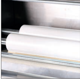
Two food-grade polyethylene rollers
