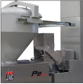
Trough flouring device Prevents the dough pieces from sticking.
